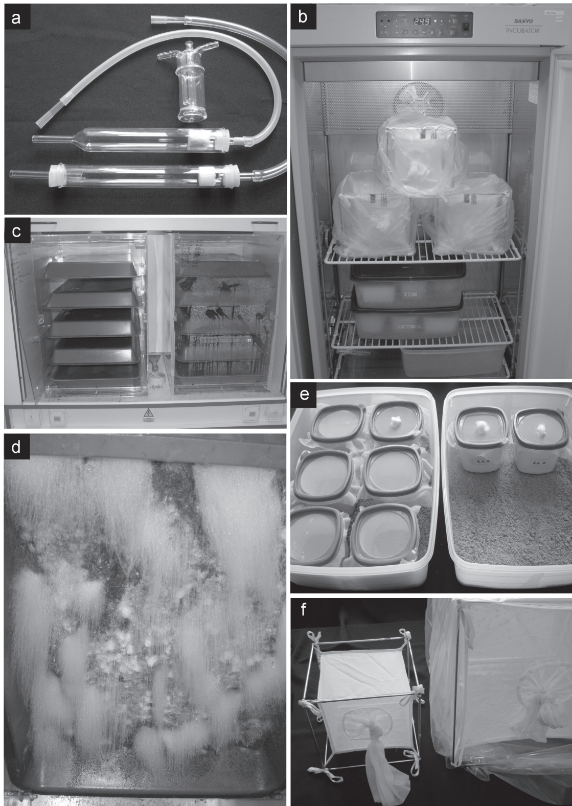
Figure 1. Equipment used for sand fly maintenance. a : two different types of glass aspirators and the glass feeder used for membrane feeding. b : boxes with larval pots and cages wrapped in plastic bags are maintained in incubator. c : two cabinets (one with front panel fitted) for fermentation of larval food. Up side down position of plastic trays ensures aerobic conditions during fermentation process. d : detail of larval food during composting process. Long, hair-like mycelia are evidence of optimal fermentation conditions. e : larval pots with a layer of plaster of Paris on sides and bottom are closed on the top with a snap cap and fine gauze. Pots are maintained in plastic boxes with a bottom filled with layer of fine sand. f : nylon cloth cages of different size are suspended on the steel frame (the larger cage here is enveloped in a plastic bag).
